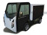
Closed cargo box in fiber with volume of 3000 litres capacity
