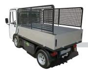
Rear bed fixed with 3 doors in aluminium and height extension in grating Dimensions: 2100x1200x365 + 710 mm
